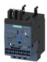
Overload relay 1...4 A Electronic For motor protection Size S00, Class 10E Contactor mounting Main circuit: Spring-type terminal Auxiliary circuit: Spring-type terminal Manual-Automatic-Reset
