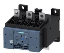
Overload relay 50...200 A for motor protection Size S6, Class 20E Contactor mounting/stand-alone installation Main circuit: busbar connection Auxiliary circuit: Spring-type terminal Manual-Automatic-Reset
