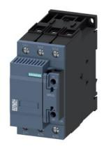
capacitor contactor, AC-6b 75 kVAr, / 400 V, 3-pole, 230 V AC, 50 Hz, auxiliary contacts: 1 NO + 1 NC, screw terminal, size: S2  $\,$
