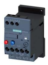
Overload relay 0.45...0.63 A Thermal For motor protection Size S00, Class 10 Stand-alone installation Main circuit: Screw Auxiliary circuit: Screw Manual-Automatic-Reset
